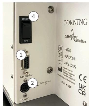
1. Connect the Touch Screen Controller cable into the rear panel of the Corning Lambda EliteMax Benchtop Pipettor.
